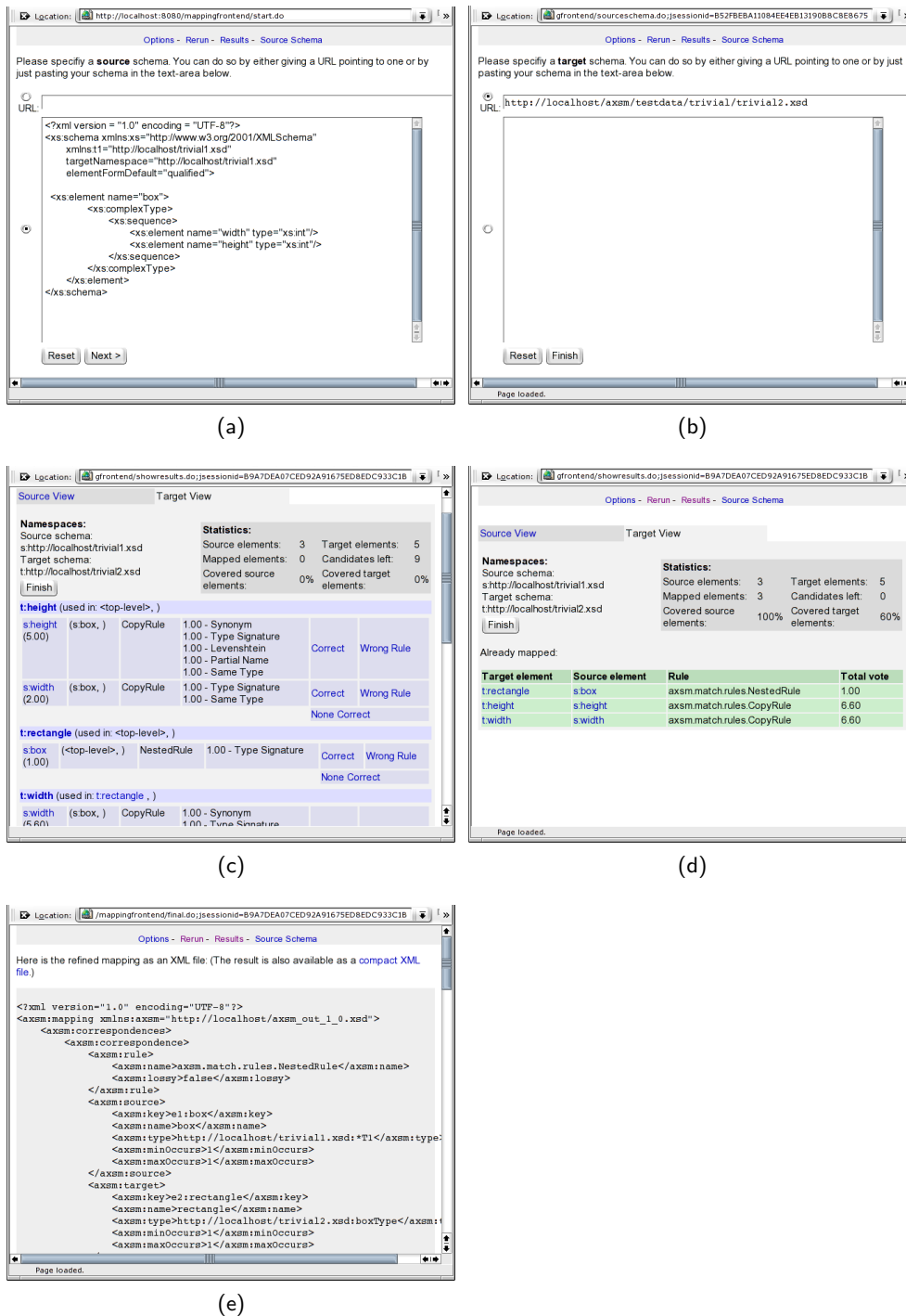
Figure 4.7: Trivial example: Screenshots. Provide schemas verbatim (a) or as URL (b), suggestions displayed (c) and after marking rectangle-box as correct (d), the final output (e).
